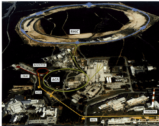
Figure 2.1: The RHIC facility as seen from the air. The circumference of the main RHIC ring is 2.4 miles.
