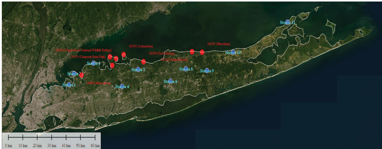
Figure 1: Map of Long Island's recorded landslide occurrences (red dots) and groundwater monitoring stations by USGS (blue dots). Blue dots represent the stations used to gather groundwater data. Stations 6 and 7 are located at the same point. These sites are located in areas of higher elevation.
