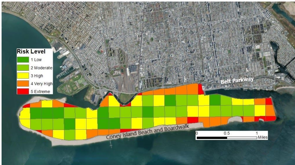
Figure 6: A GIS classification map that presents area flood rate in terms of the risk level. Risk level was described with five risk levels starting from low risk (level 1; green color) to high risk (level 5; red color).
