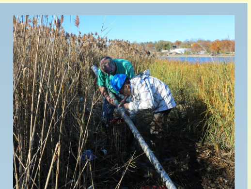
Figure 2: Sediment coring in the Douglas Manor wetland.
