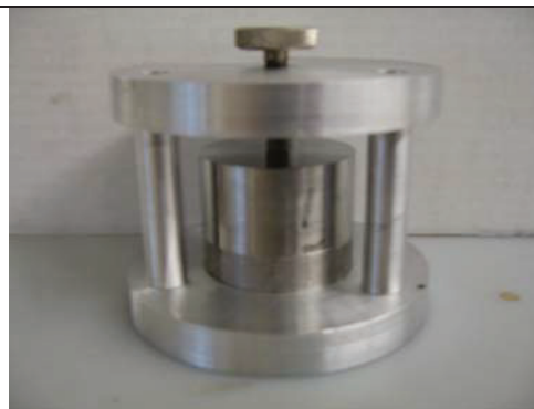
Figure 2: Vacuum press used to press patterns using pressure onto thin films
