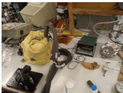
Pressure chamber (left), laser (bottom left), voltmeter (right), high pressure crosses (bottom right).
